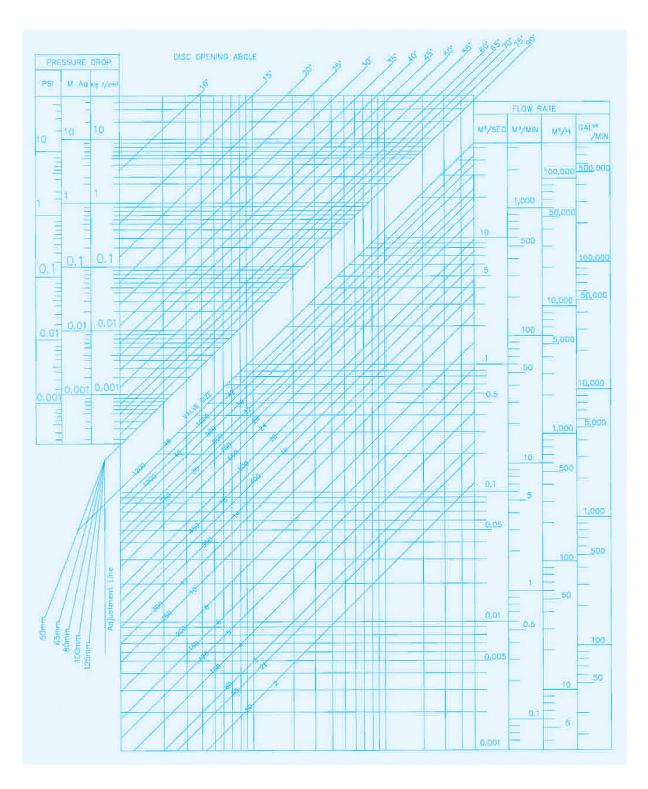
The curve on the left shows the relationship between valve opening and rate of flow at a constant pressure differential. Generally Butterfly Valves are most suitable for controlling flow but are not recommended for flow control where the valve opening is below  $30.(\text{Ideal: }30^{\circ}\text{ to }70^{\circ})$
